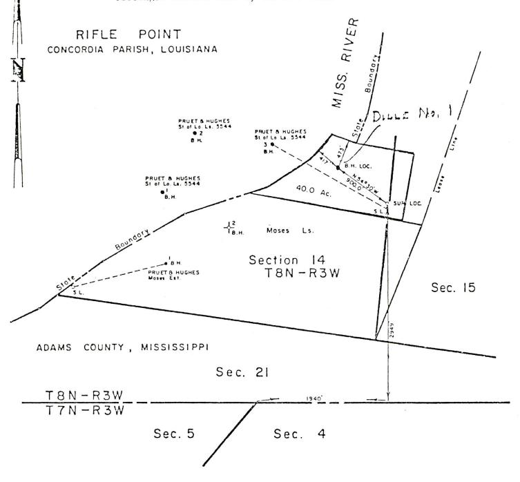
DESCRIPTION OF LOCATION: From the most easterly corner of Section 5, T7N-R3W, Adams County, Mississippi, go East along the north boundary of T7N-R3W for 1940 feet; thence North at right angles for 2949 feet to surface location in Section 14, T8N-R3W; thence N 54° 30' W for 900.0 feet to bottom hole location.
