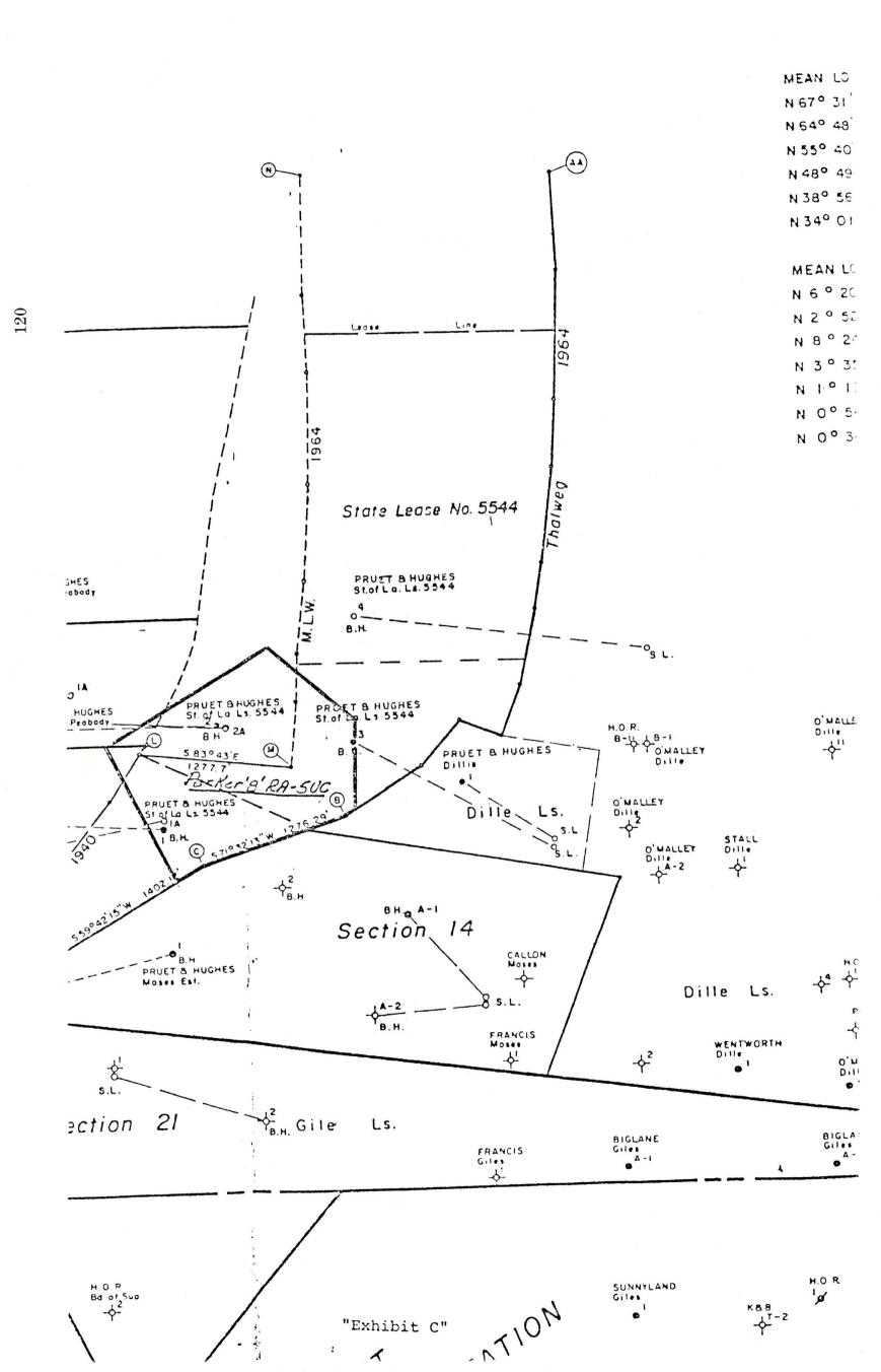
NOTE: The drilling unit shown hereon lies totally within the confines of a rectangle 2314.46 feet by 1094.44 feet.
