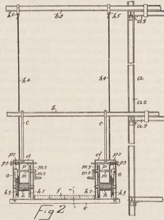
single idea, "the idea of supporting the scaffold to outriggers by means of auxiliary bars or rods," so that the platform or scaffold by the lengthening of the cables can be raised to a greater height than before. In other words, the assertion is that Murray invented nothing and saw nothing in his device but means of raising the scaffold, and, to use counsel's word, all other "functions" were
