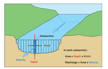
**Figure 3.** Current-meter discharge measurements are made by determining the discharge in each subsection of a channel cross section and summing the subsection discharges to obtain a total discharge.
