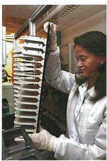
A contractor assigned to the Terrorist Explosive Device Analytical Center loads sample plates into the mass spectrometer.
