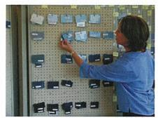
A forensic examiner in the Laboratory's Chemistry Unit searches the paint panels of the National Automotive Paint File; the panels are cataloged according to their color.
