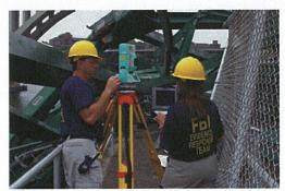
ERT personnel assisted in the aftermath of the Minneapolis bridge collapse by providing advanced site documentation using laser transit surveying systems.
