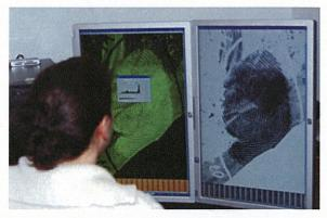
A latent print examiner uses the Latent Print Digital Imaging System to improve the quality of a latent fingerprint submitted to the Laboratory.
