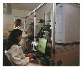
Contractors assigned to the Terrorist Explosive Device Analytical Center prepare sample plates for mass spectrometry analysis.
