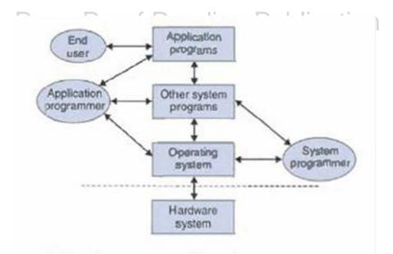
J. Garrido & R. Schlesinger, Principles of Modern Operating Systems 8 (2008) ("Figure 1.4. An External View of a Computer System").
