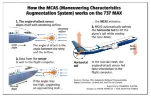
119. Further compounding its negligent design of MCAS, Boeing submitted documentation to the FAA indicating that MCAS could move the horizontal tail a maximum of 0.6 degrees, which described the first iteration of MCAS, not the second iteration that would ultimately be used on all 737 MAX delivered to Boeing customers, including Lion Air, Ethiopian Airlines and Southwest.
