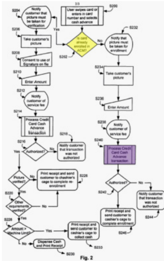
Figure 2 of Sanford illustrates a method for conducting PIN-less credit card transaction in a flow diagram. Ex.
