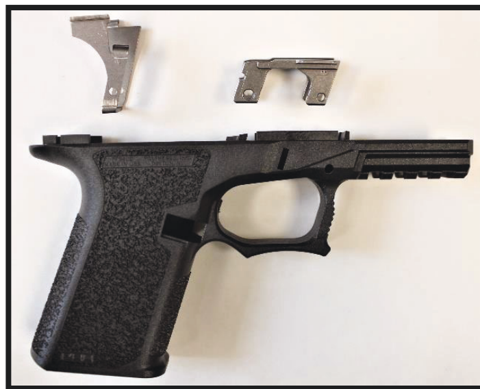
Polymer80 partially complete frame with Locking Block Rail System and Rear Rail Module – “Temporary Rails” present
