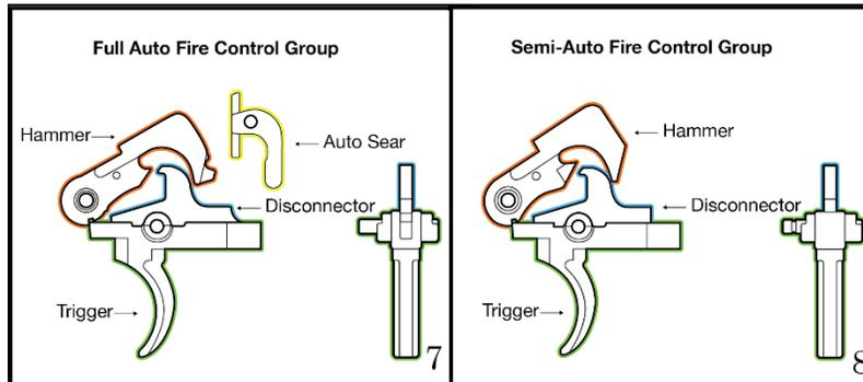
For a true machinegun, the “hammer follow” problem is one of precise timing. If the hammer is released too early, the hammer will follow the bolt and the firearm will not fire, needing to be manually re-cocked. Too late, and the bolt will lose forward travel before tripping the mechanism. This issue of timing is handled in machineguns by an “auto sear.” Image 7.
