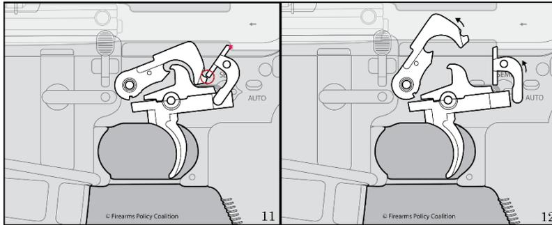
Thus, a machinegun equipped with an automatic fire mechanism contains a “self-acting or self-regulating mechanism,” which upon simply keeping the trigger depressed, without any further input, will “self-actuate” and “regulate” itself to fire successive rounds without “hammer follow.” Machineguns, and the other automatic firing devices that fall within the statute’s wording, are incomparable to bump stocks in their function.
