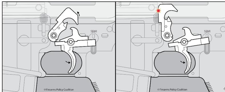
When the trigger is actuated, the trigger sear slides out of the way of the hammer, allowing the hammer to swing, ultimately striking the firing pin. Image 4.
