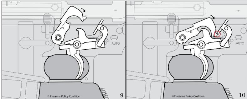
When a machinegun is set to fully automatic mode, the semi-auto disconnecter is disengaged and the “auto sear” engaged. Image 9. The “auto sear” is precisely designed and regulated to hold the hammer in the
