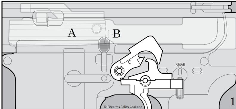
At the core of a self-loading firearm is the bolt. Image 1(A). The bolt ensures that an ammunition shell stays firmly in place so that sufficient energy pushes the bullet down the barrel, rather than simply pushing the bolt rearward. In a single-shot or manually repeating firearm, the bolt stays firmly locked in place during firing, whereas a self-loading firearm uses some of the energy from the fired round to cause the bolt to reciprocate.
