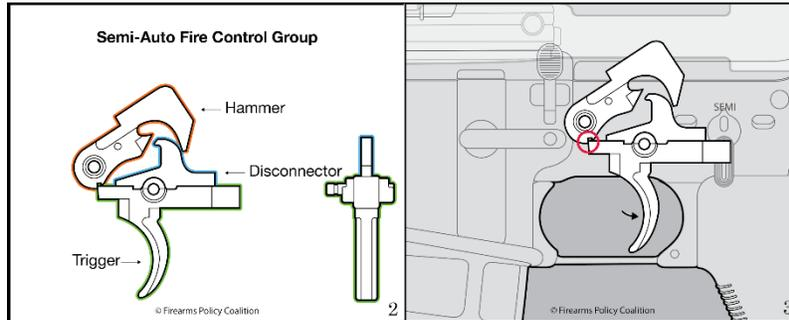
The trigger mechanism of a semi-automatic firearm consists of a trigger, hammer, and disconnector. Image 2. The hammer is spring-loaded, storing energy as it is moved rearward into the “cocked” position. The trigger keeps the hammer in the “cocked” position by way of its “sear,” a geometric plane locking the two pieces together. Image 3.
