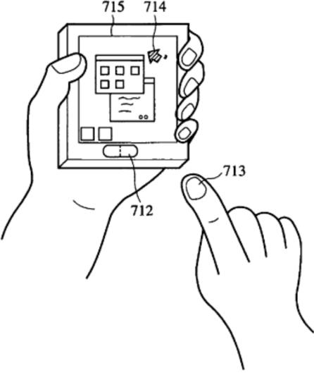
Figure 78 shows "a compact portable information device" having "a size that can be held by one hand." *Id.* at 52:5–8. The device includes a window (712) for a lighting unit and a photo-detection sensor unit. *Id.* at 52:12–14. Numazaki describes controlling the position of a cursor (714) on a screen by moving a finger (713) in front of the window (712). *Id.* at 52:14–16.
