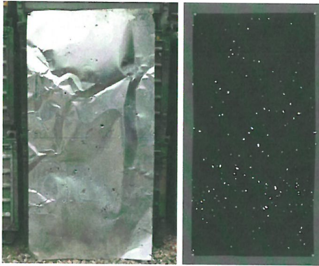
Fig. 2. Typical witness plate after test (left) and after preparation for evaluation (right).
