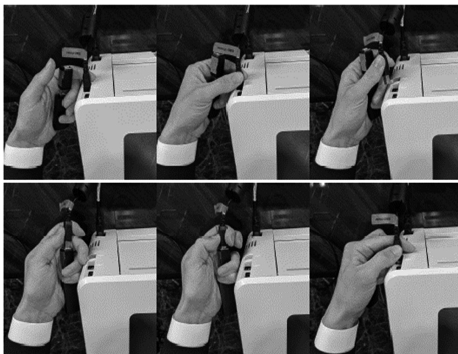
Figure 12: Installing Malware in the Polling Place. An attacker can install vote-stealing malware on the ICX by attaching a small USB device for under two minutes. This sequence shows me reaching behind the printer, unplugging the cable that leads to the BMD, and connecting the device to the end of the cable.
