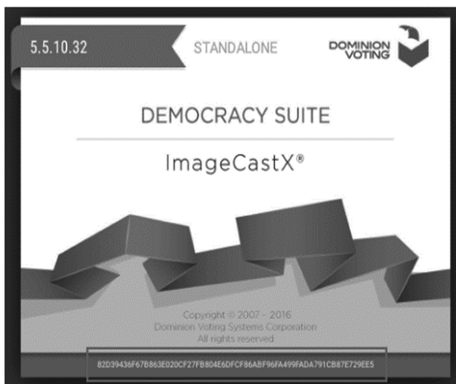
Figure 8: Defeating Hash Validation. The ICX App displays the SHA-256 hash of its APK on the screen, as shown here. However, this behavior is controlled by the app itself, so a maliciously modified app can simply show the expected hash value instead of its real one, thereby avoiding detection.
