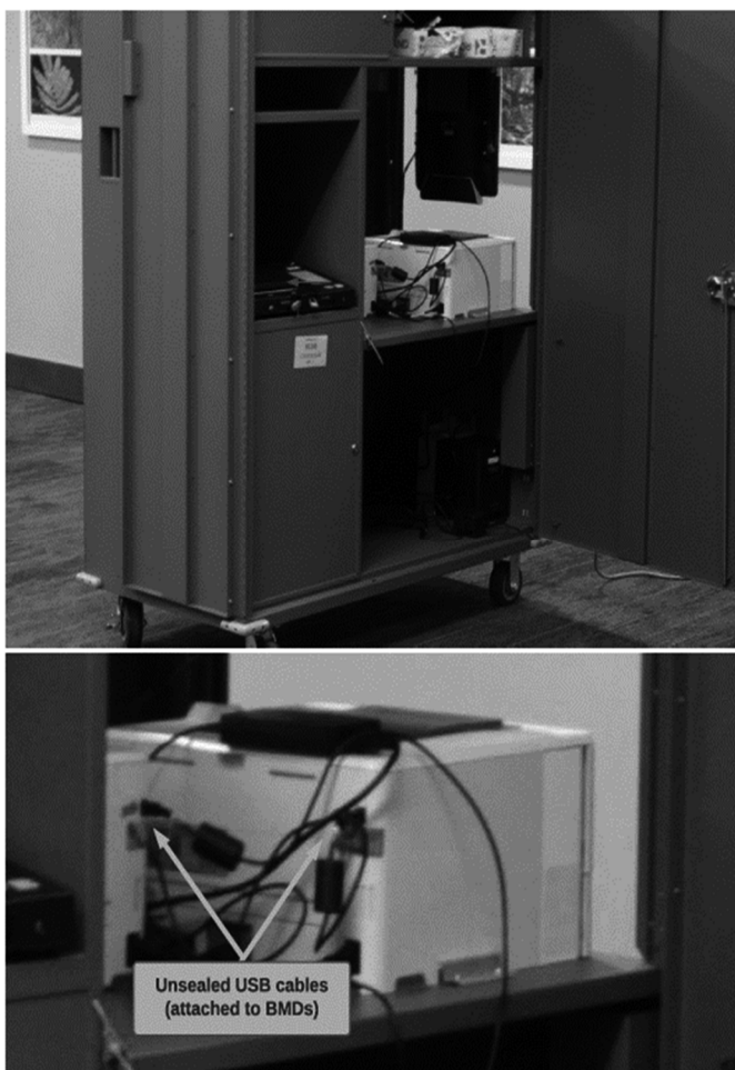
Figure 9: ICX USB Interfaces are Exposed to Voters and Unsealed. A USB cable connects the BMD to an off-the-shelf laser printer. At polling places, the end of the cable attached to the printer is physically
