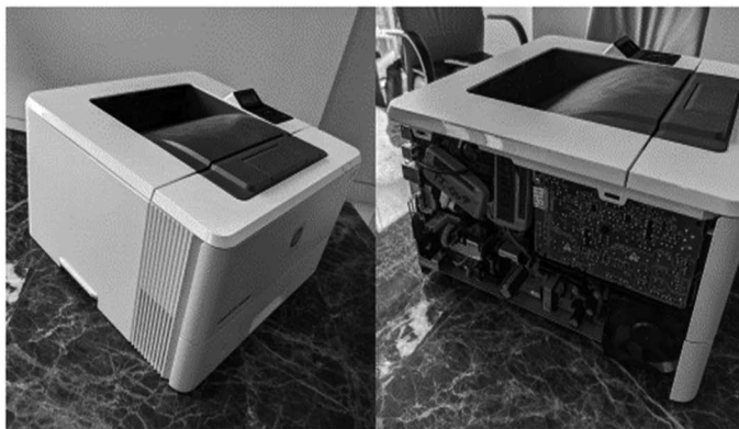
Figure 4: Demonstration Malicious Hardware. I developed a hardware-based attack that modifies data sent from the ICX to the printer, altering ballot QR codes to change recorded votes. The attack device (the two red modules seen in the right photo) is completely hidden inside the printer's plastic housing. Similar malicious hardware could be added in the supply-chain or while in storage.
