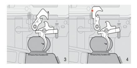
In a semiautomatic firearm, the bolt re-cocks the hammer. By the time the bolt reciprocates, the operator may still have the trigger depressed. This is where the "disconnector" comes into play. When the trigger is depressed, the disconnector moves into its active state. Image 5. When the weapon fires, the bolt travels rearward, pushing the hammer to the rear. The disconnector captures the hammer near its rearmost position. Image 6.
