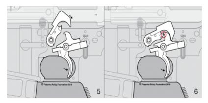
Then, as the user releases the trigger, the hammer slips off the disconnector and back onto the trigger's sear, where it is ready to be fired again. Image 7.
