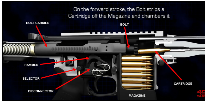
Figure 2: Post-Fire Forward Motion of Bolt Carrier 9
