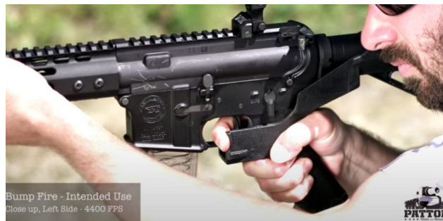
Figure 2: After the first shot, the shooter's finger rests against the extension ledge of the bump stock, which "constrains" the recoil and the opposing forward force so that the firing unit slides in a linear direction, propelling the firing unit against the stationary finger, causing the firing cycle to repeat.
