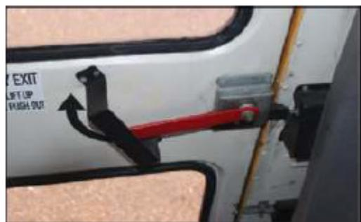
To open the emergency exit, a person must unlatch the door by pulling the red lever upward, and then push against the door.
