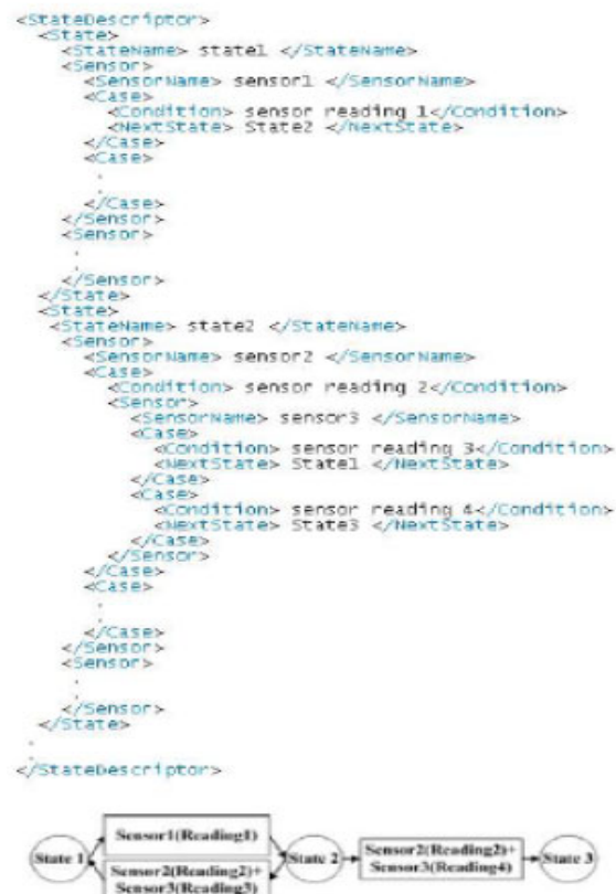
Figure 1: The format of XML based state descriptor and its implication of state transition.
