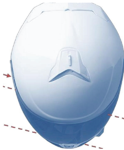
EXHIBIT NO. 3: Approximate trajectories of the three pellets that struck the helmet based on corresponding exit defects.
