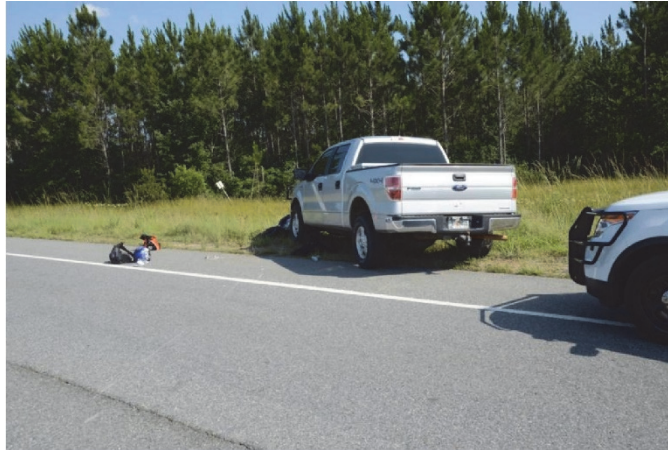
EXHIBIT NO. 8: Eunice's unmarked truck where it came to rest on top of the motorcycle. You can clearly see from the gouge marks that confirm Schantz's direction of travel was toward the shoulder of the road. Also, the road in that area is clear of any sand or gravel that would have caused Eunice to slide when he braked. Furthermore, there are no brake or skid marks showing a sudden stop.
