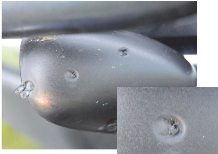
EXHIBIT NO. 4: The three pellet strikes to the right mirror. A close-up of the middle defect clearly shows an angled glancing strike with no penetration.
