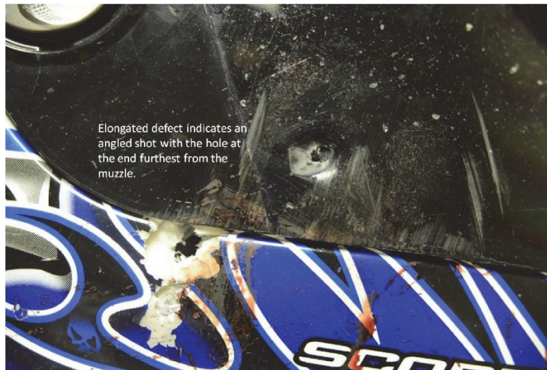
EXHIBIT NO. 2: Elongated pellet defects confirm angled shot.
