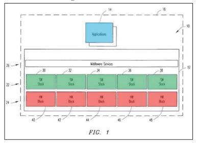
Non-native application software (blue) is installed, loaded, and run on the mobile platform. *Id.* at 4:14-16. The software services component (green) provides services such as control, structured storage, and access to hardware driver software. *Id.* at 5:33-40. The hardware com-
