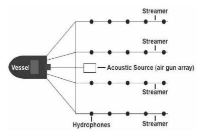
J.A. 20254. If there is a cross-current, the streamers may drift and become offset from the towing direction of the vessel. This phenomenon is known as "feathering." The extent to which the streamers become offset from the towing direction of
