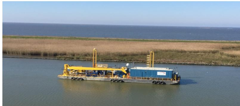
The 60' yellow crane has a 30-ton capacity and is permanently attached to the barge.<sup>4</sup> It is shown in its horizontal position lowered from the bow on the left side of the image toward the stern on the right. The OB 808 can navigate to customer sites in navigable water as shallow as “two to four feet in depth,” as well as to sites located in the deeper navigable waters of the Gulf of Mexico. The onboard crane allows Crescent to “reach
